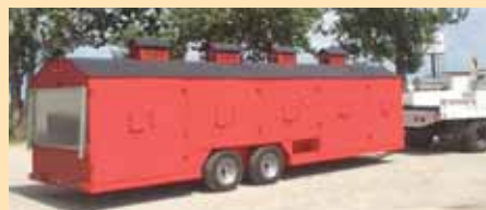
Giant cooker is built on a tandem axle trailer and measures 24 ft. long. On top are four 14-in. sq. metal cupolas, painted red with black cupolas on top.
