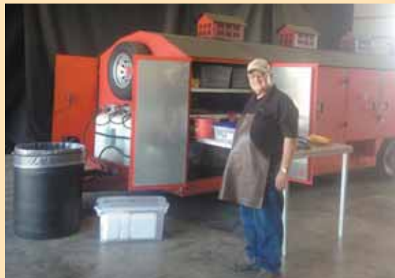
Giant cooker is built on a tandem axle trailer and measures 24 ft. long. On top are four 14-in. sq. metal cupolas, painted red with black cupolas on top.
