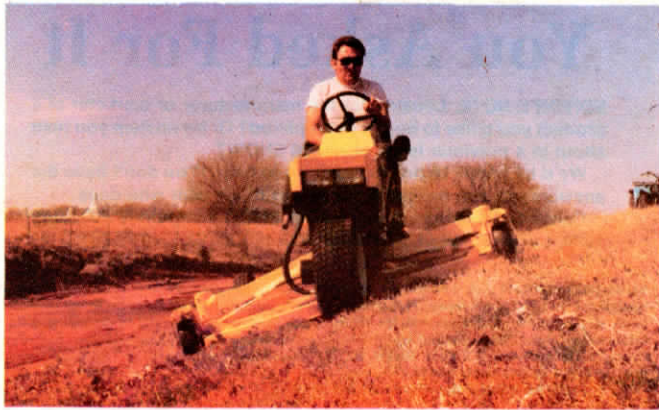
Independently floating decks on either side handle slopes at angles up to 30°.
