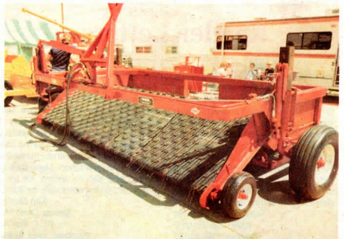
Rake's easy-handling finger pickup moves hay into windrows with virtually no leaf loss. Can also be used on small grains.
