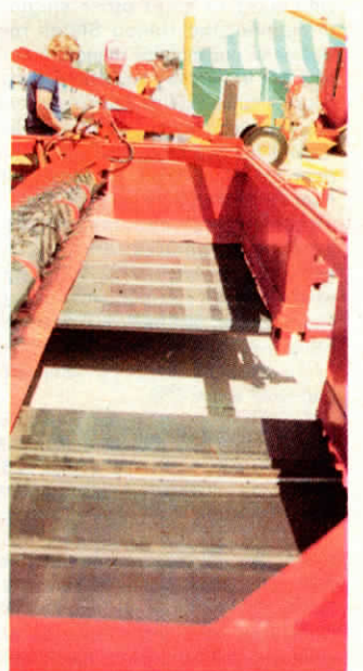
Rear cross conveyor drops hay, or grain, into windrow at center.
