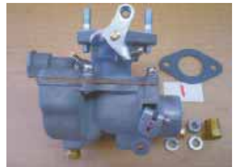
Mike Finch restores Farmall Cub and Cub Lo-Boy carburetors to "better than new" condition. Photo shows new choke shaft and lever with cork top-to-bowl gasket.
