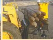
Floyd Yoder's skid loadermounted fence post driver works fast, hammering posts like a jackhammer at 800 blows per min. Unit's domed hammer handles wood, steel, pipe and T-posts equally well.
