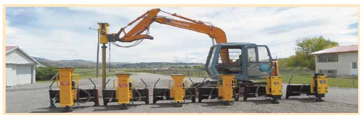
Montana Post Drivers are available in several sizes, starting with a 500-ft. lb. model. They can now also be fitted with mounts for excavators.
