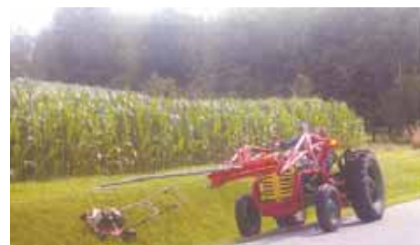
Side-mount hitch carries a 22-in. wide push mower about 10 ft. beyond the bucket on James Rohr's loader tractor. Chains attached to mower deck allow it to roll easily over uneven ground.
