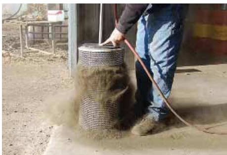
During tests on a pair of Deere 7750 tractors, one tractor’s air filter was cleaned once a day. Nearly 5 lbs. of dirt was removed daily and the tractor used 58 gal. less fuel per day than the tractor with the dirty filter.
