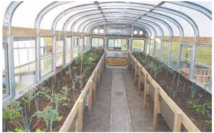
They started by removing all the bus's passenger seats. On the larger bus they replaced the entire tin roof with clear poly.
