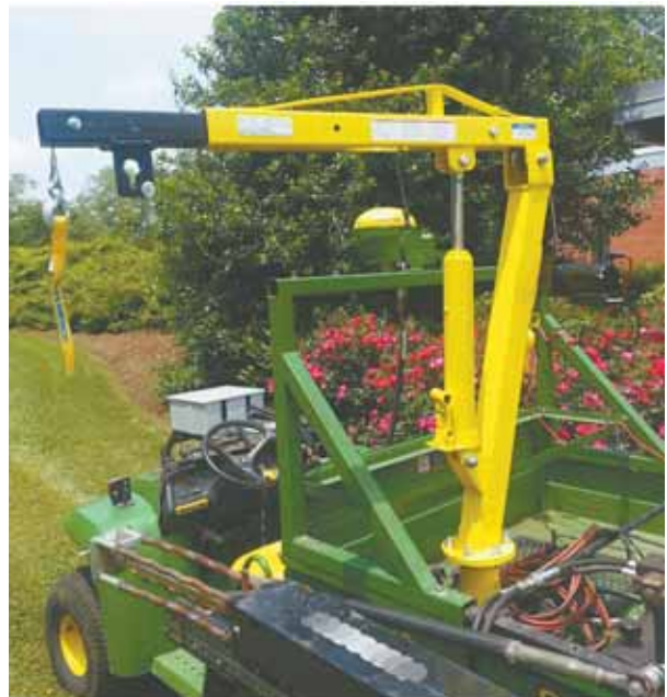
Jib crane mounted in bed of utility vehicle comes in handy for lots of jobs around the farm, says Gary Roberson at North Carolina State University.
