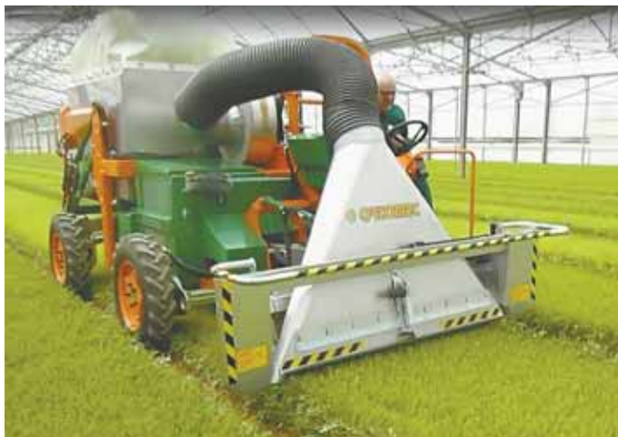
Self-propelled machine vacuums away clippings and other debris from commercial scale beds of greens, making it easier to get a second cutting without having to replant.
