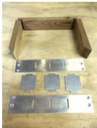
Soil blocker was built from scrap cedar wood and has an aluminum metal frame.
