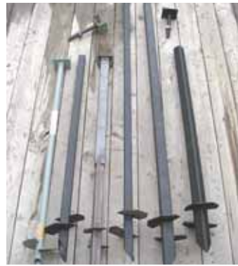
Drivable posts made from square tubing have a flat blade welded on at an angle at bottom that “screws” into the ground.
