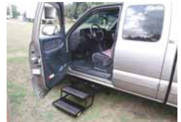
Bottom step folds down to about 1 1/2 in. above the ground, creating a small set of stairs.
