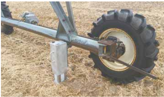
Battery-powered Easy Jack offers a much safer way to change tires and gearboxes on center pivot irrigators, and also can be used for other jobs.
