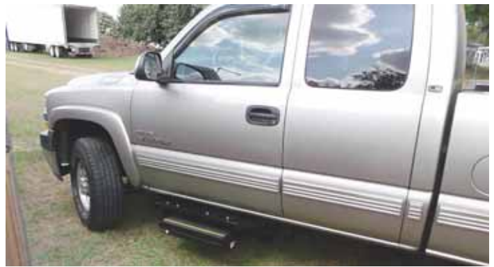
Darrell Hartzog replaced the driver’s side running board on his mother’s pickup with electric-operated, retractable steps that he bought from a local RV dealer.
