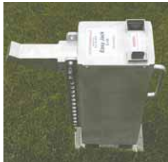
Steel arm on one side does the lifting. Operator pushes a 2-way switch on top of jack to make it go up or down.
