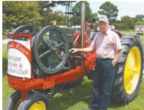
**Tom Shell replaced the engine on his Massey Harris 30 tractor with a McCormick-Deering "hit and miss" engine. It powers a hydraulic pump that runs a hydrostatic motor mounted on the transmission shaft.**
