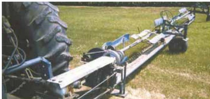
Gerald Gould couldn't justify the expense of a large rotary mower to cut his 25 acres of CRP land, so he built this 20-ft. sicklebar with a belt-driven reel.
