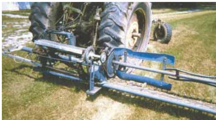
The reel was made from 1 1/2-in. dia. pipe with batts cut from plastic barrels.
