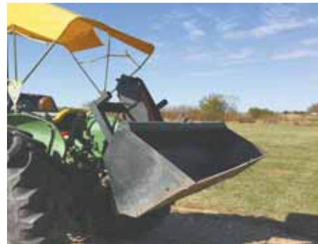
Ron Vogelsmeier modified a 6-ft. wide front-end loader bucket to fit his tractor's 3-pt. hitch.
