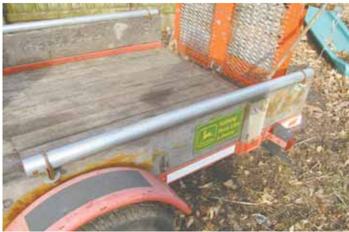
Garage door springs inside pieces of conduit on the side of Nichol's utility trailer make it easy to raise the rear drive-on tailgate.
