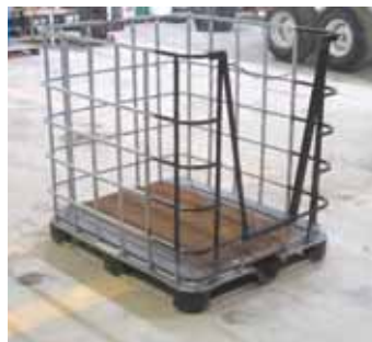
Forklift-mounted “safety cage” was built using the metal cage off a 250-gal. chemical shuttle. Inventor David Hansen bolted a plywood section onto the shuttle floor and then bolted expanded metal onto the plywood.
