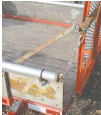
The spring-assisted cables run through pulleys to tailgate ramp.
