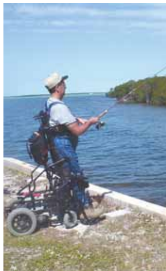
Ed Bell gets around and even goes fishing in his own Standing Company wheelchair - an electric chair with a manual control for standing.
