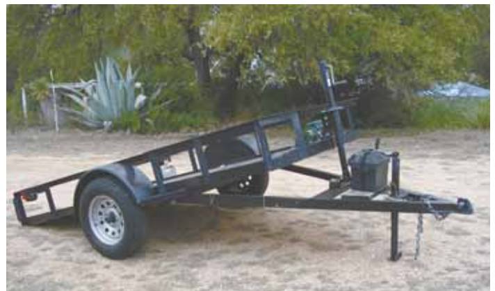
Glenn Thompson bought a trailer equipped with a tilt bed and mounted a winch and screw-jack on front.
