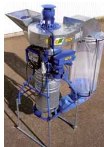
Polish-built Sosnowski seed cleaner uses centrifugal force to remove trash from all types of seed.
