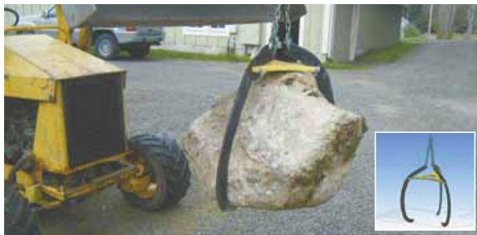
Rock Claw can handle big boulders with no problem. Three steel arms with curved points at their lower end are connected to a lift chain.
