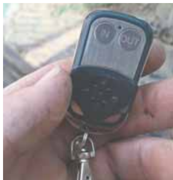
Jared Rasmussen made life easier for his dad by installing remote control on a Haybuster's discharge auger. The remote activates a 2-way solenoid to raise and lower the auger.
