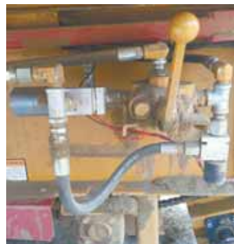
Jared Rasmussen made life easier for his dad by installing remote control on a Haybuster's discharge auger. The remote activates a 2-way solenoid to raise and lower the auger.
