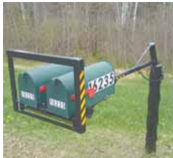
Steel tube frame protects mailboxes. An angled mounting pin allows arm to swing freely, yet return to center.
