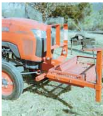
Front receiver hitch can be fitted with an L-shaped bracket that supports a vice and an expanded metal basket, or various hitches can be inserted.
