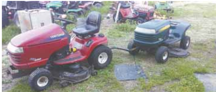
Zach Jensen replaced rear mower's rear transaxle with the front steering axle off another riding mower, facing it backward. In effect, the rear mower has 4-wheel steering which allows it to do a better job of following.
