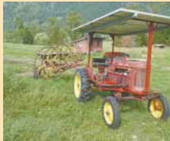
Drew Gailius converted this old Massey Harris tractor from gas to solar, replacing the engine with a 48-volt DC motor and transmission. Three 250-watt solar panels mount horizontally on an overhead frame.
