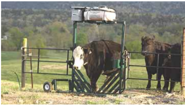
Solar-powered fly sprayer is designed to be placed in a gateway. It automatically sprays insecticide onto cattle without causing stress to the cattle or operator.
