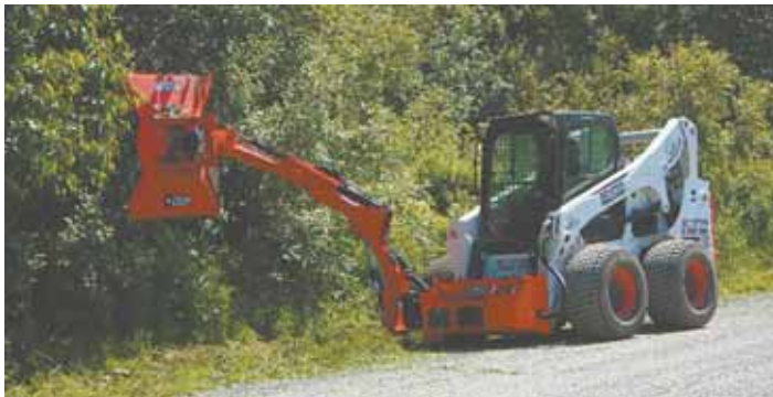
Skid loader-mounted 48-in. rotary mower can rotate up to 180 degrees, making it ideal for heavy roadside clearing.
