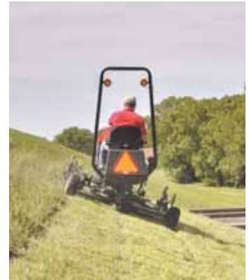
Auto-leveling system on hillside mower keeps engine and control platform upright on steep slopes.
