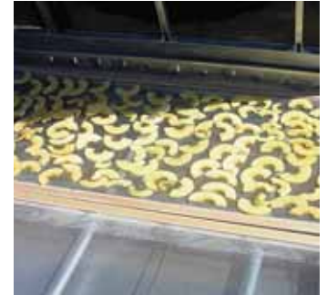
Sunlight shines through clear twin-wall polycarbonate glazing and heats up black-painted aluminum sheet metal, which radiates heat to the food below it.
