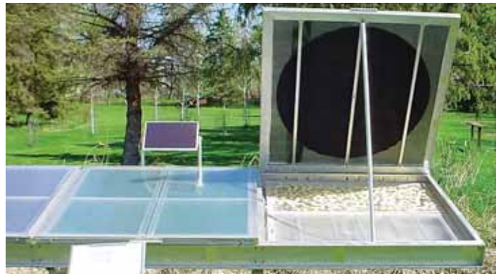
Dehydrator measures 12 ft. long by 4 ft. wide and is built in 3 sections. Each section has a pair of hinged doors for access.
