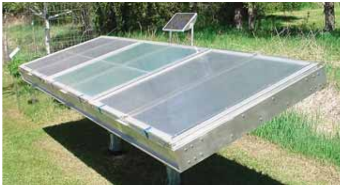
Solar food dehydrator is built almost entirely from scrap aluminum. "I built it because I wanted a more energy efficient dehydrator that can turn large quantities of apples into chips that we can sell," says Kent Scheer.
