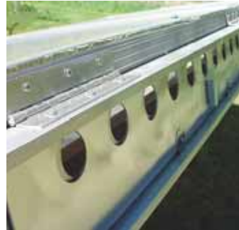
Sunlight shines through clear twin-wall polycarbonate glazing and heats up black-painted aluminum sheet metal, which radiates heat to the food below it.
