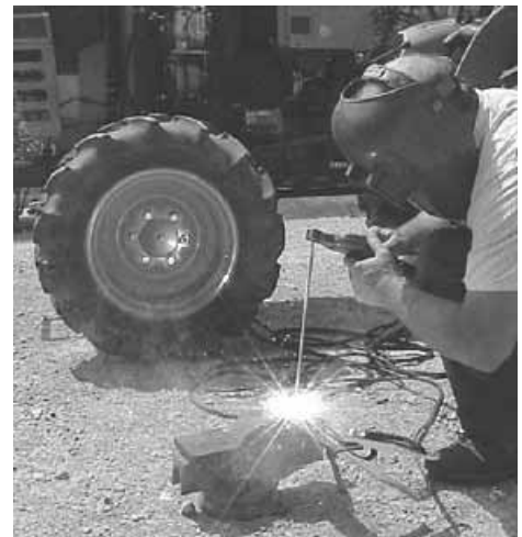
Remote controls are built into the electrode holder so you don’t need to go back and forth to your welder to readjust power.
