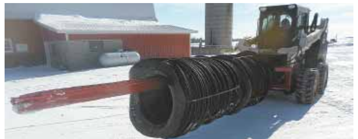
A track and chain is used to move tires on and off unit's 16-ft. steel boom. Boom raises up to a 20-degree angle.
