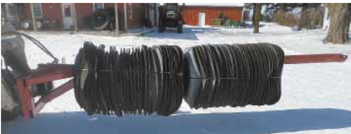
Skid loader-mounted "shooter" works great for putting tires on silage piles and bunkers, and for loading and unloading tires on trucks and trailers.
