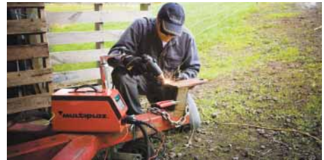
Not much bigger than an old-time radio, all the Multiplaz 3500 welder needs is 110 or 220-volt current, water and alcohol.
