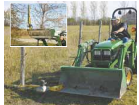
Hydraulic-powered cutter attaches to loader bucket.
