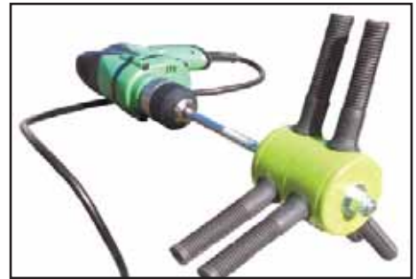
Drill-powered Power Plucker uses multiple rubber fingers to remove feathers without damaging skin or meat.
