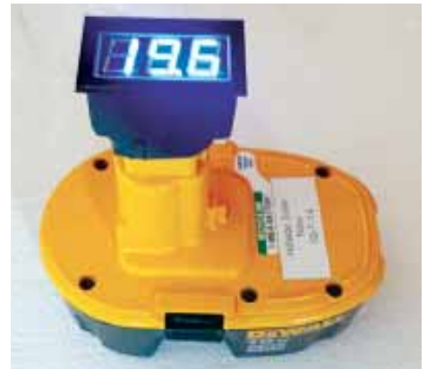
Digital battery tester attaches to the posts on any DeWalt 18-volt battery and shows the voltage in big, brightly lit numbers on top.
