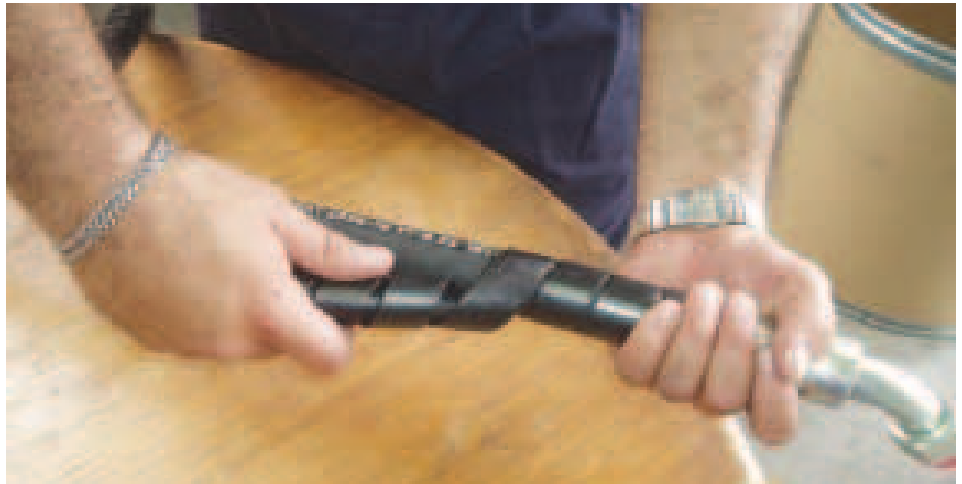
HoseSaver wraps provide protection for hydraulic hose as well as wires and cables. Raguse also sells a canvas wrap, below left. He built the machine that cuts plastic pipe of different sizes.
