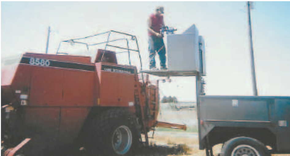
Portable workbench mounted on back of Schoenenberger's 2-ton service truck lifts up to 9 ft. in the air.
