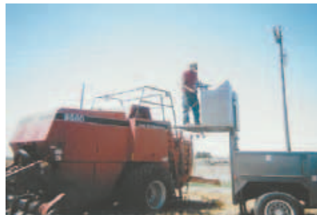
Forklift mast is used to lift a workbench. Fold-down platform provides a place to stand.
