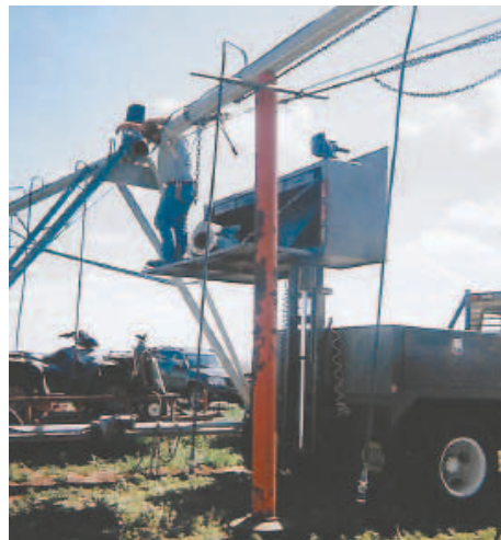
Forklift mast is used to lift a workbench. Fold-down platform provides a place to stand.
