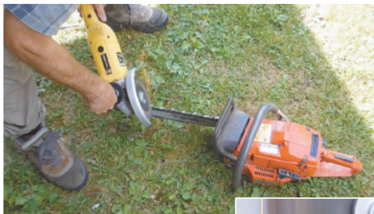
Matthias Wandel uses an angle grinder with a cutoff wheel to quickly sharpen chainsaw chains.
