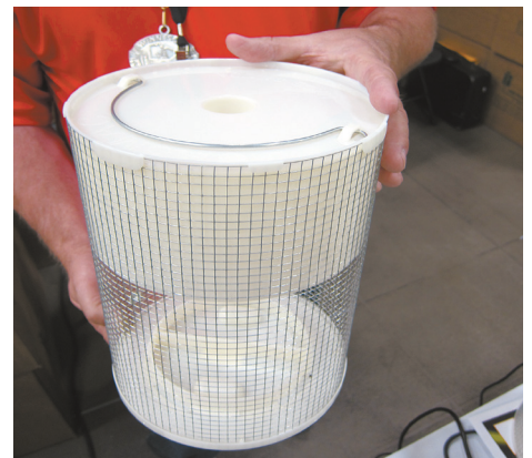
Mouse climbs up trap's mesh sides and jumps through an entrance hole at top. To release the mouse you remove a plastic tray at bottom.
