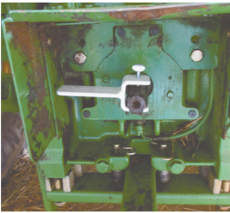
Y-shaped wrench turns pto shaft with enough leverage to easily line it up to implement.
