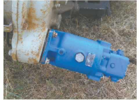
Marty Winchell bought a cement mixer with no truck. He drives it with a new hydraulic drive that hooks up to the hydraulics on his tractor.
