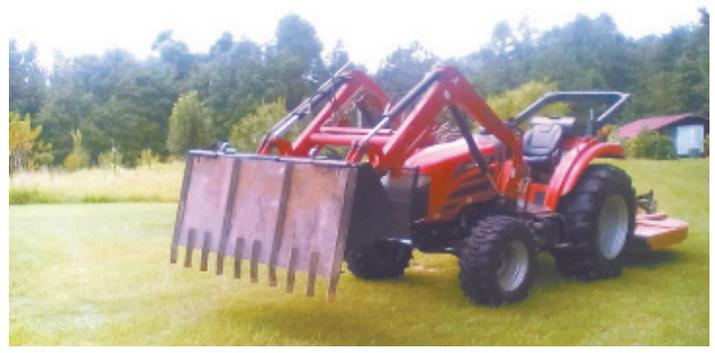
Bucket-mounted dirt blade lets Ledbetter blade dirt without getting dirt in bucket. It can be quickly popped off so bucket can be used to lift and load material.
