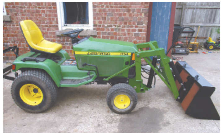
Steve Nichols built this "new and improved" mini loader that's designed to fit Deere's 425, 445 and 455 garden tractors.
