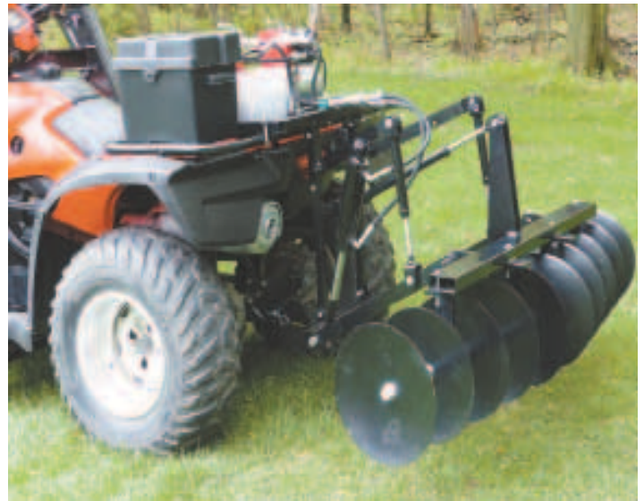
Some of the Wild Hare accessories available include this rear 3-pt. hitch and 57-in. disk harrow, as well as a battery box.
