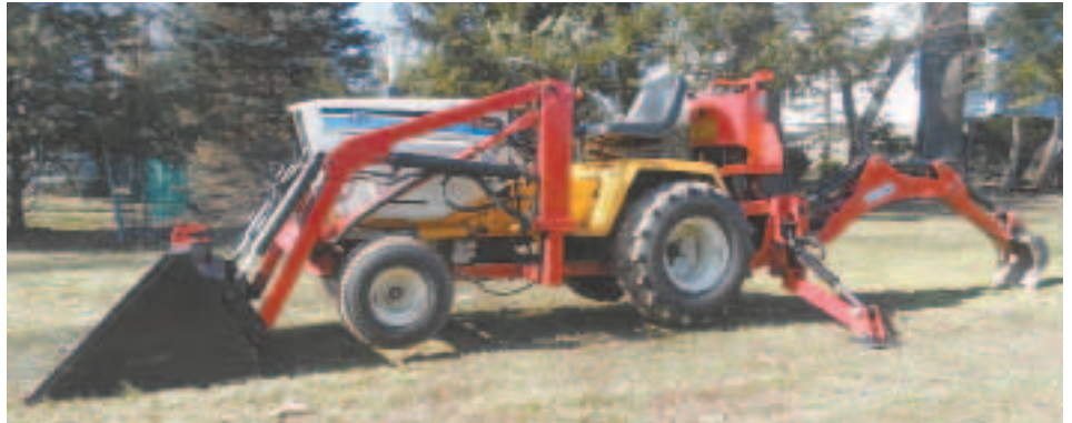
"It amazes me every time I use it," says Ken Esposito about the loader/backhoe he built out of a Cub Cadet garden tractor.
