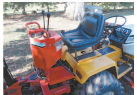
When Esposito wants to use the backhoe, he just flips the seat around and goes to work.
