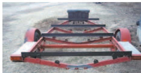
John Drew built a 6 by 14-ft., 2-wheeled flatbed trailer out of a used boat trailer. He spaced four 3-in. angle irons across the frame and welded them in place.
