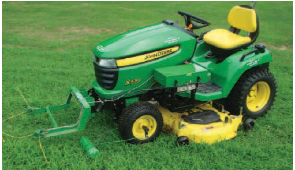
Riding mower has 2 coil sensors mounted on front, one on each side. Sensors follow underground wire and send information to an electronic box, which in turn operates a motor that's used to control mower's steering system.
