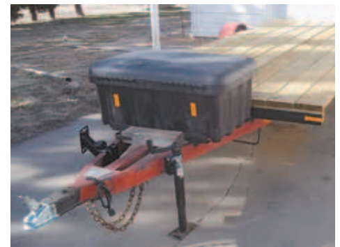
John Drew built a 6 by 14-ft., 2-wheeled flatbed trailer out of a used boat trailer. He spaced four 3-in. angle irons across the frame and welded them in place.
