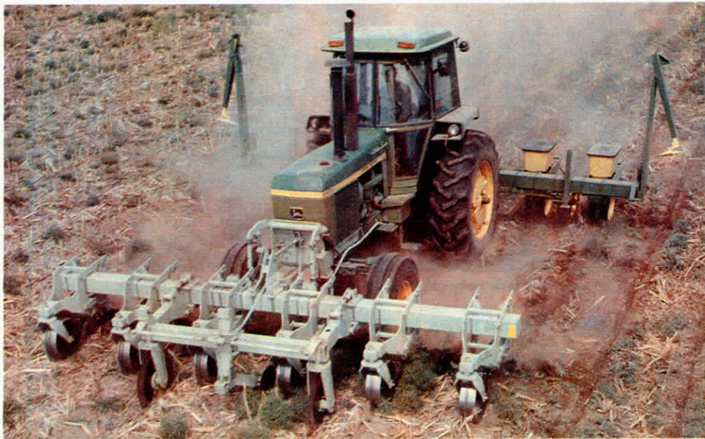
Injector knives can be mounted on the Ridge Rider attachment for injecting fertilizer or anhydrous.
