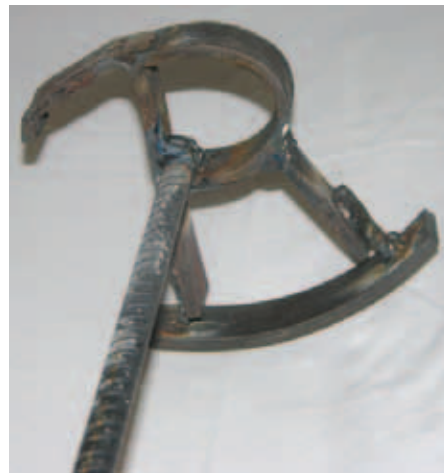
Farmer Ken Summa’s patented branding iron made with a Multiplaz welder.
