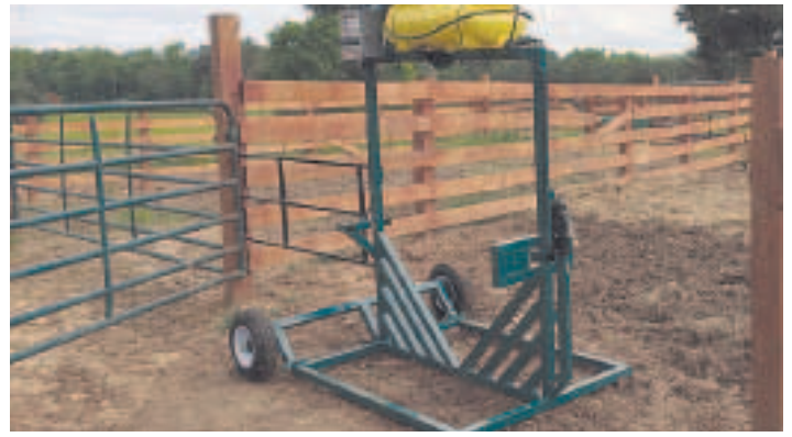
Self-contained sprayer comes mounted on a 2-wheeled dolly that tows behind any vehicle equipped with a 2-in. ball.
