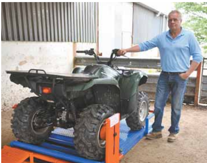
Anti-theft device uses the motion of the ATV’s rear wheels moving forward to send a piston through one of the rear wheels, locking vehicle in place.
