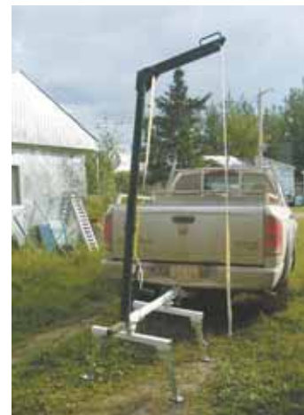
Home-built crane slips into receiver hitch to load a trailer or pickup bed. For heavy lifts, a stable base with legs is attached.
