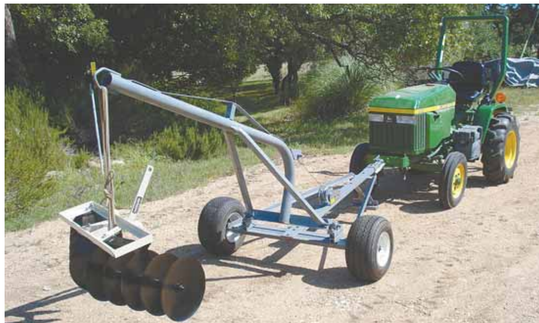
Glenn Thompson mounted an old 3-pt. mounted crane on wheels and hooks it up to a ball hitch on his Deere compact tractor. "Works great to move garden tractors and their implements around on my farm," he says.
