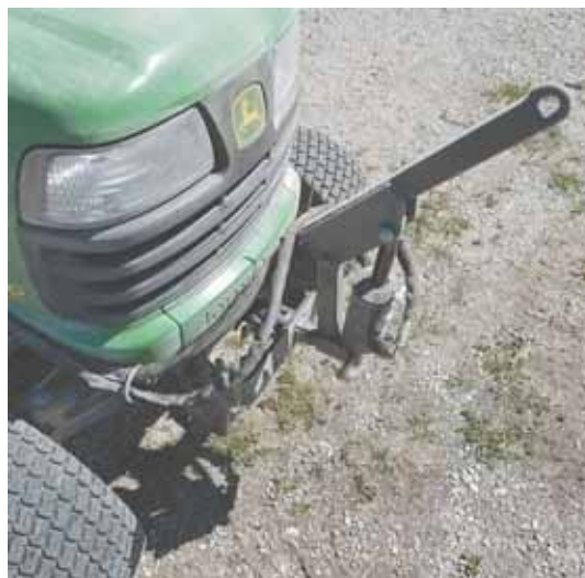
Rick Robinson turned the front-mount manual lift on his garden tractor into a hydraulic-operated power lift, by using the tractor's receiver hitch.
