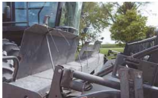
Metal deflector has a 4-in. lip at a 30-degree angle on top to deflect flying beans back into combine auger.
