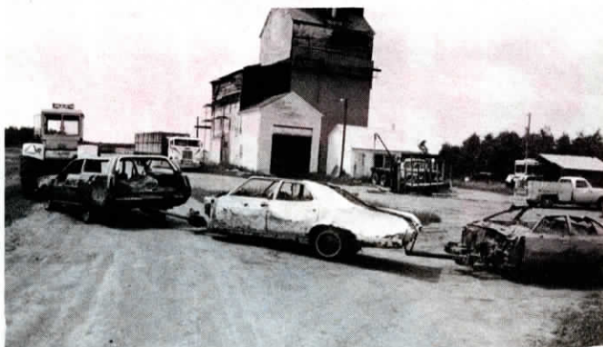
Digney removes front ends of all cars except the one directly behind the tractor, allowing him to make nearly 180° turns with several feeders in tow.
