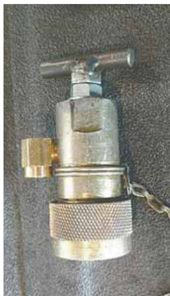
Releasing pressurized hydraulic couplers is as easy as turning a bolt.
