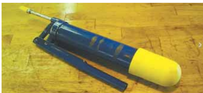
Grease gun cap slides over barrel of grease gun and collects grease drips. It also acts as a priming bulb and dust cover.
