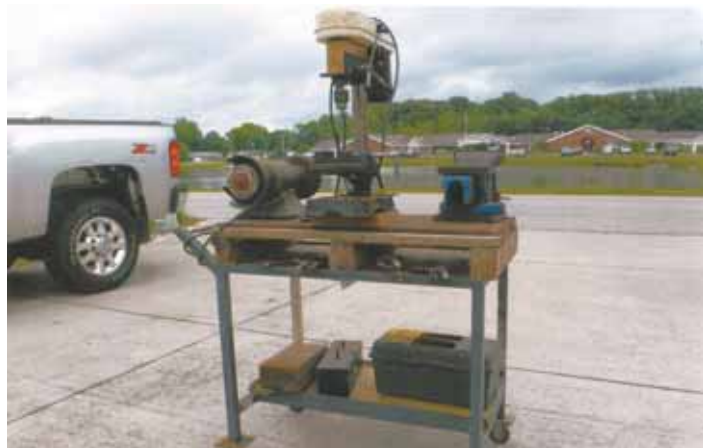
Gene Williams mounted a grinder, drill press, and vise on a 4-wheeled cart fitted with caster wheels, making it easy to move them in and out of his garage.
