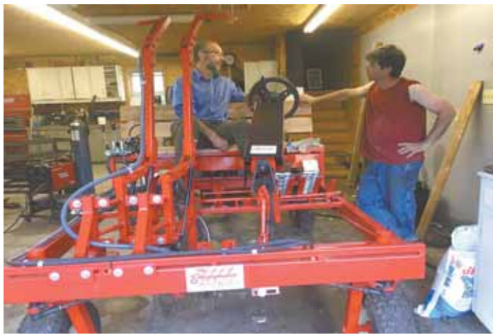
David Greenberg built his self-propelled cultivator from a 19 hp. Kubota zero-turn mower. The lightweight machine produces minimal compaction.
