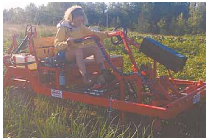
Operator moves handle levers back and forth as needed to weed crops.
