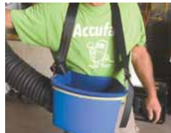
Phil Brown's self-propelled vacuum apple picker now comes with picker-carried baskets so pickers don't have to place apples in a trough at the end of the tubes.
