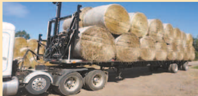
Any large flatbed trailer can be fitted with the Exclerator bale system that quickly secures loads with steel cables on both sides of trailer.
