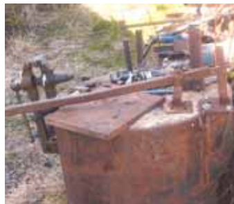
Solid outdoor workbench was made from a 3-ft. length of 4-ft. dia. steel pipe filled with concrete and gravel.
