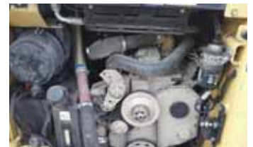
Melvin Zook repowered his 2012 Volvo skid loader with an inexpensive, used Cummins diesel. "I had to fabricate motor mounts for the engine. Everything else worked out great," he says.
