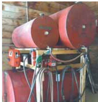
Tim Renger saved space inside his shed by building this wood rack that holds 3 big tanks.
