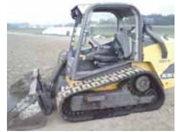
Melvin Zook repowered his 2012 Volvo skid loader with an inexpensive, used Cummins diesel. "I had to fabricate motor mounts for the engine. Everything else worked out great," he says.
